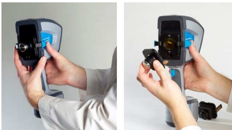
Figure 10 Removing the sampling interface
