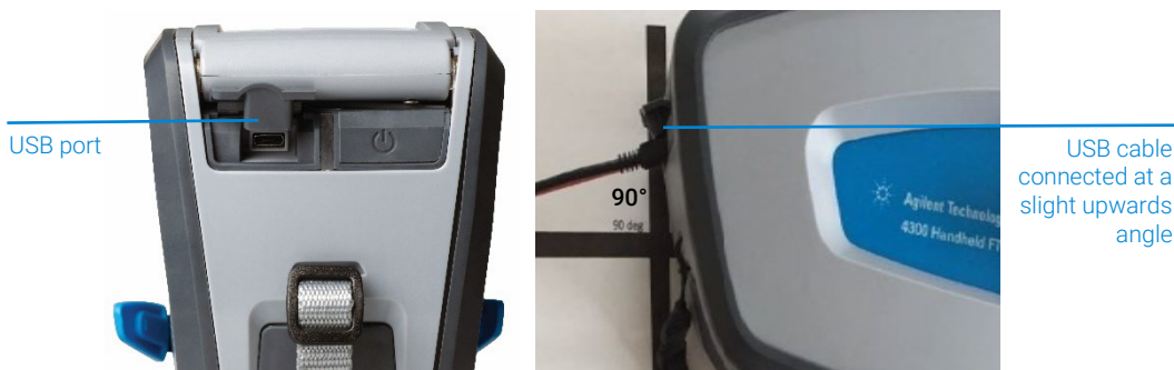
Figure 7 USB port (Left) & USB cable connected to instrument (Right)
